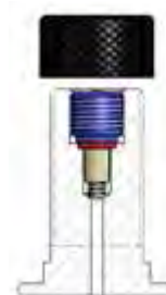
Model of valve stem integrated 5/8" 18 UNF (D)
