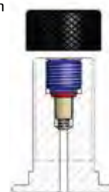
Model of valve stem integrated 5/8" 18 UNF (D)
