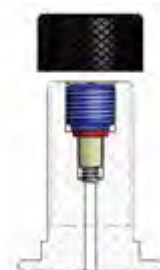
Model of valve stem integrated 5/8" 18 UNF (D)
