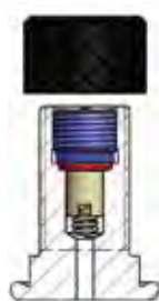
Model of valve stem integrated 7/8"14 UNF (C)
