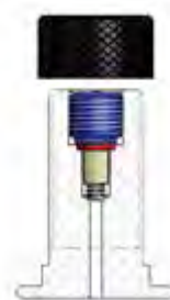
Model of valve stem integrated 5/8" 18 UNF (D)
