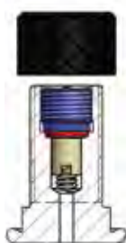
Model of valve stem integrated 7/8" 14 UNF (C)
